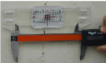
For more accurate monitoring, Vernier, Dial or Digital Calipers can be used to measure the distances between the monitoring spigots. The distance between the spigots is recorded on the record card supplied with each Tell-Tale.
